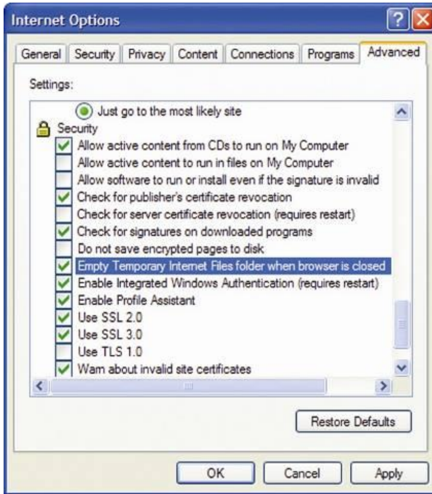
Figure 1-22 Set Internet Explorer not to keep a cache after the browser is closed
