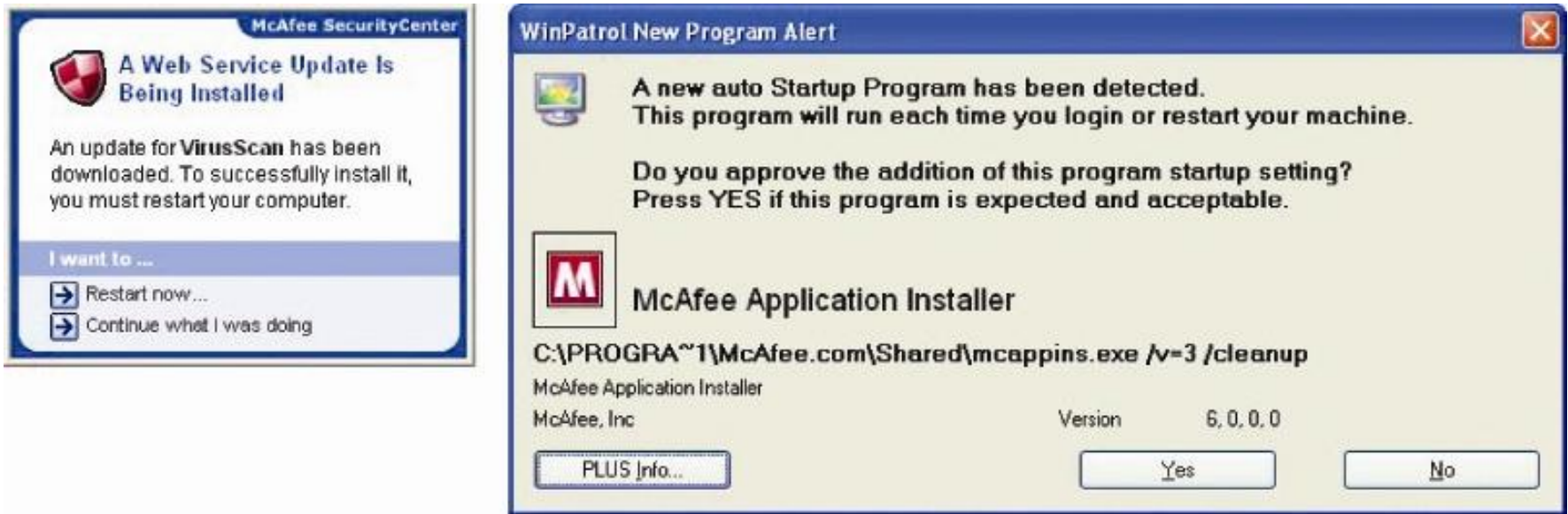
Figure 2-46 WinPatrol by BillP Studios alerts you when the startup process has been altered
